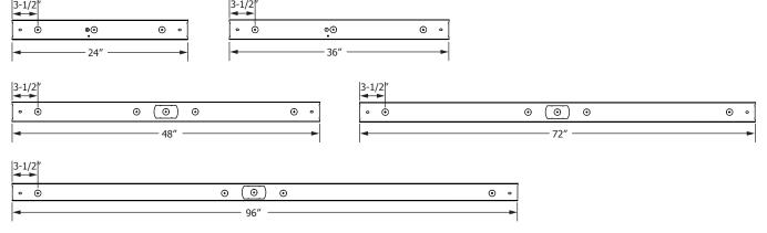
Double KO for easy wiring of the unit, 4ft or larger units.
